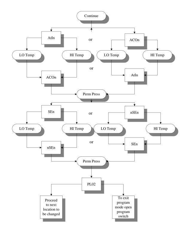
Display will read coin/time accumulation status. I.E. "AtIn" accumulative time or "ACOn" accumulative coin. If no change, press "Perm Press" key, otherwise press "HI" or "LO" key and then press "Perm Press" key.
