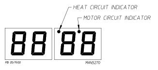
The L.E.D. indicator dots located at the top portion of the display indicates the various microprocessor controller (computer) output functions while a cycle is in progress. These dots do not necessarily mean that the outputs are functioning. They are only indicating that the function (output) should be active (on).
