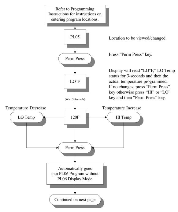
Summary: LO Temp is programmable from a minimum of 100° F to a maximum of 190° F in ten-degree increments or from a minimum of 38° C to a maximum of 88° C in five-degree increments.
