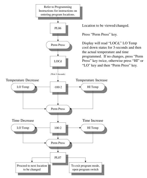
Summary: Cool down temperature is programmable from a minimum of 70° F to a maximum of 190° F in ten degree increments or from a minimum of 21° C to a maximum of 88° C in five-degree increments.
