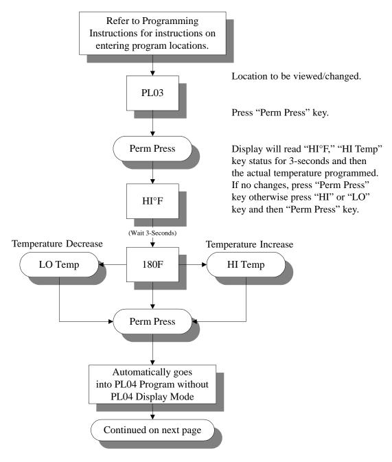
Summary: HI Temp is programmable from a minimum of 100° F to a maximum of 190° F in ten-degree increments or from a minimum of 38° C to a maximum of 88° C in five-degree increments.
