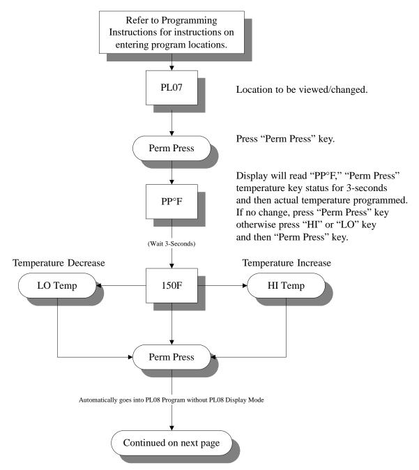
Summary: Perm Press Temp is programmable from a minimum of 100° F to a maximum of 190° F in ten-degree increments or from a minimum of 38° C to a maximum of 88° C in five-degree increments.
